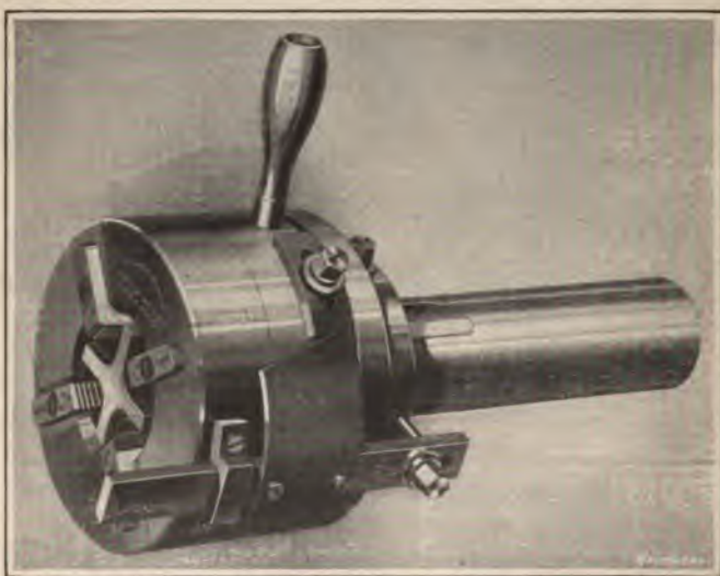
Fig. 31. Geometric Taper-threading Die of Inside Trip Type
